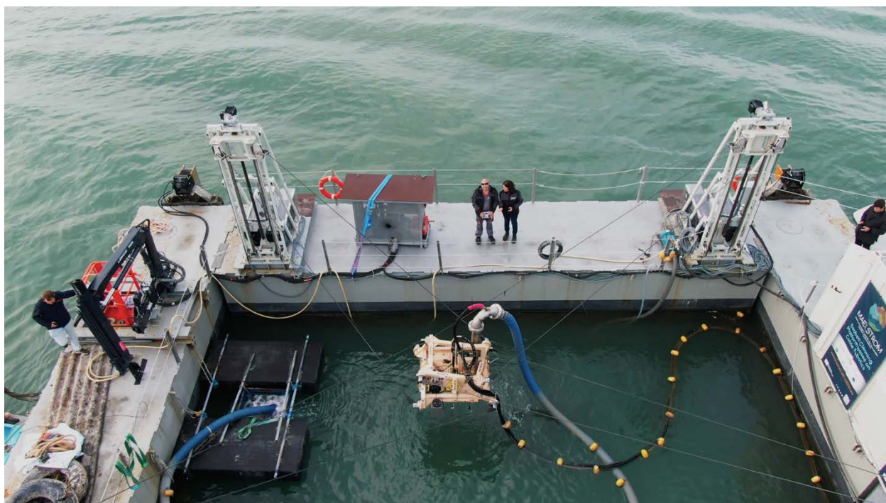
Robotic platform for cleaning the seabed – EU H2020 MAELSTROM project
